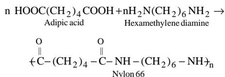
It has high tenacity and elasticity. It is resistant to abrasion and not affected by sea water. It is used for reinforcement of rubber tyres, manufacture of parachute, safety belts, carpets and fabrics.
